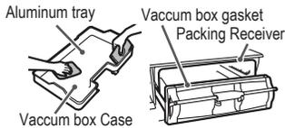
3. Assembly the Vacuum Box case attach with the core of Vacuum Box Door.
